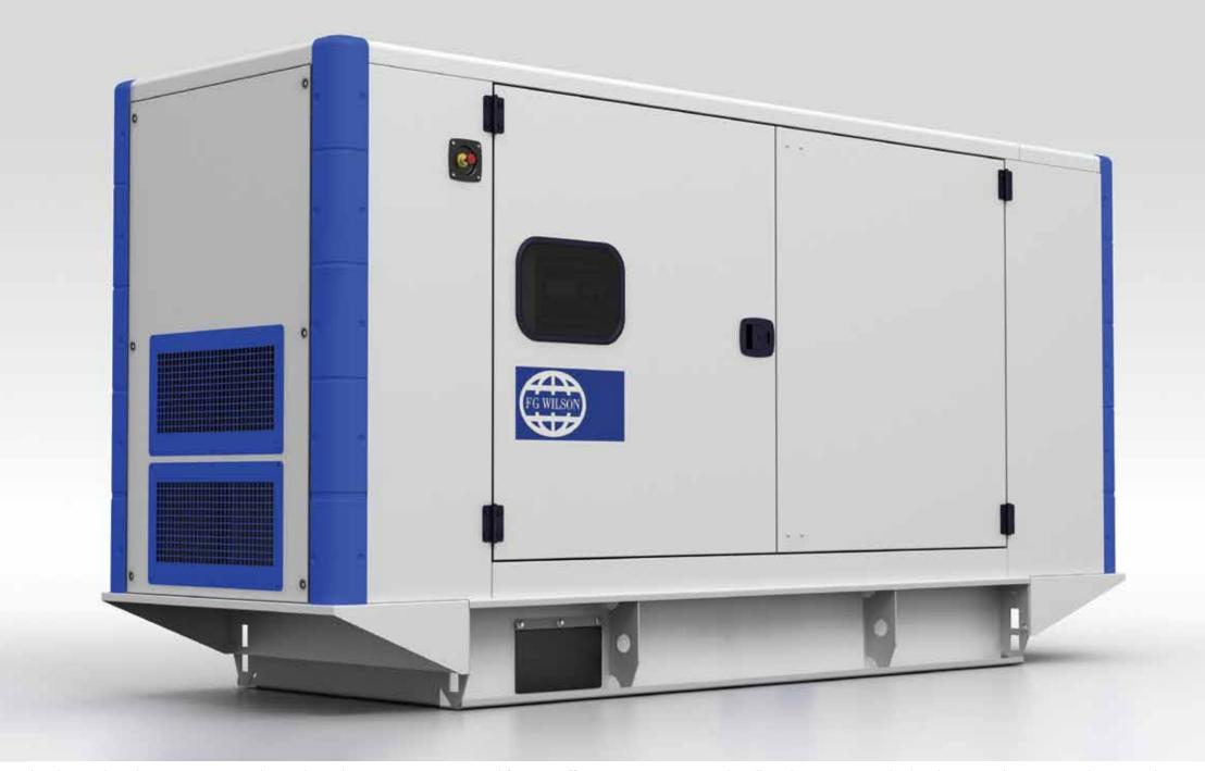
A galvanised steel construction, an advanced powder coat paint process and features offering protection against handling damage as standard make our enclosure range the most robust in its class. A base frame which extends beyond the enclosure reduces handling damage, whilst side-hinged doors enhance maintenance access and hook latches ensure operator safety by preventing unintended closure. Access for radiator cleaning and maintenance is through easily removed end panels.
