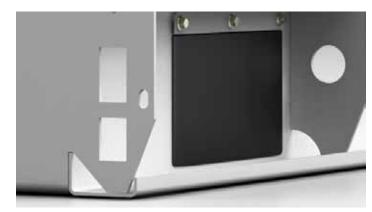
A removable gland plate offers ample cable access for a bend radius of 8 times the outside diameter of single core cable (up to 300 mm diameter), whilst preventing rodent access.
