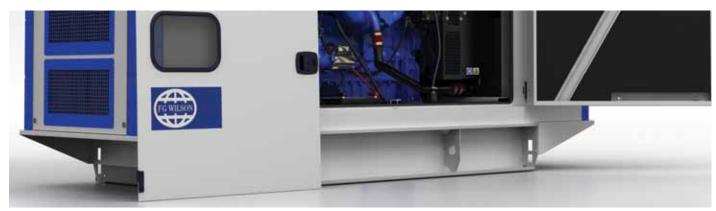
Lift-off hinges allow doors to be totally removed, even at an angle of 45°, facilitating service in the most confined installation spaces. Side-hinged doors on each side of the enclosure allow access to the control panel whilst the generator set is running.
