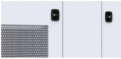
Rotation compression latches ensure a flush door seal with the enclosure frame preventing water ingress; while sloped door seals and purposefully designed grill cut outs ensure optimal water run off.
